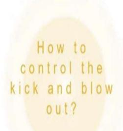
> the kick can be controlled by increasing the mud density to be greater than the formation pressure.
