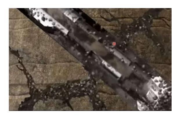
To solve this problem we add special materials to the mud, so these materials could close the holes or fractures that causes the lost circulation zone.
