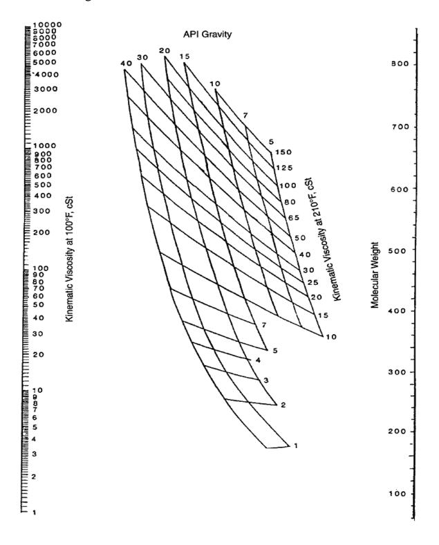
To use this figure, based on the value of  $v_{38}$  a point is determined on the vertical line, then from  $v_{99}$  and SG, another point on the chart is specified. A line that connects these two points intersects with the line of molecular weight where it may be read as the estimated value.
