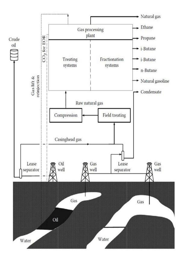
Figure 1: Schematic Overview of Natural Gas Industry.
