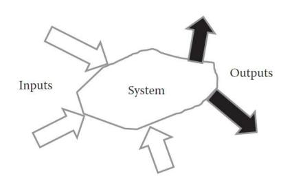
$\begin{cases} \text{Rate of } X \\ \text{into the system} \end{cases} - \begin{cases} \text{Rate of } X \\ \text{out of the system} \end{cases} = \begin{cases} \text{Rate of accumulation} \\ \text{of } X \text{ in the system} \end{cases}$
