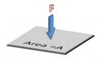
Figure 2.1. Definition of pressure. Force F acting on an area of A m<sup>2</sup>.
