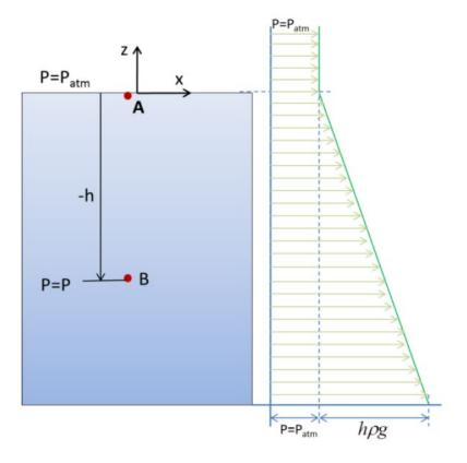
Figure 2.4. Pressure variation in the direction of gravity
