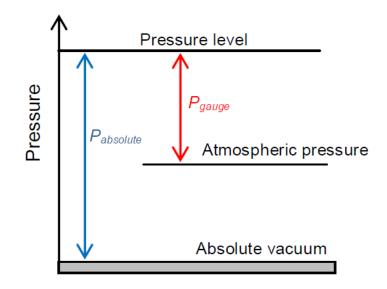
Figure 2.5. Relationship between gauge, absolute and atmospheric pressures.
