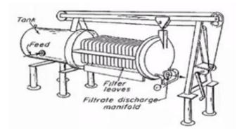
A set of vertical leaves is held on a rack. During the operation leaves are inside the closed tank. Feed enters through the side of the tank, filtrate passes through the leaves into a discharge.
