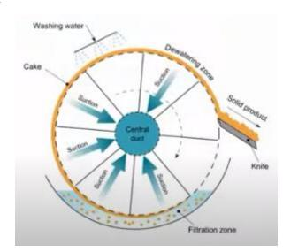
A horizontal drum with slotted face rotates at 0.1 to 2 RPM in an agitated slurry trough. A filter medium cover on the outer surface of the drum which is partially submerged into liquid.
