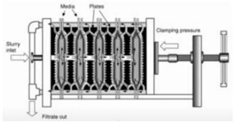
Consist of plates and frames arranged alternately. Plate having ribbed surface and frame is hollow provide space for filter cake. Filter clothes are placed over each plate on both sides.
