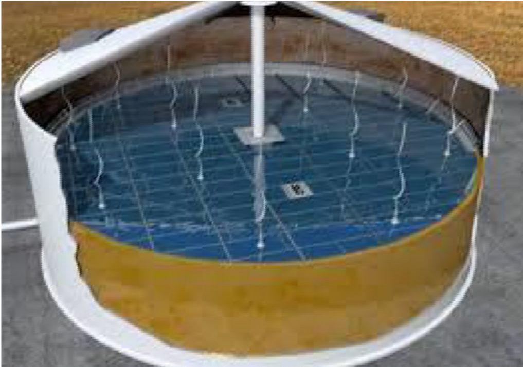
Internal floating roof
