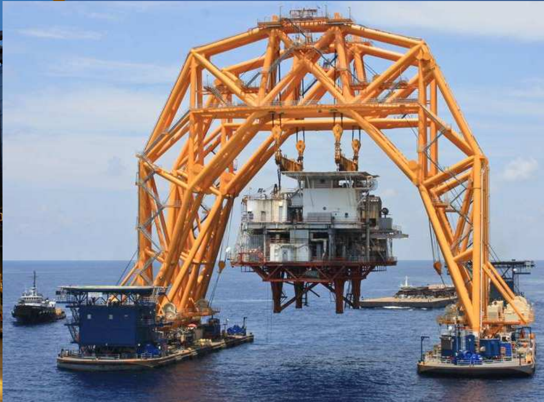
Special vessel to remove offshore platform
