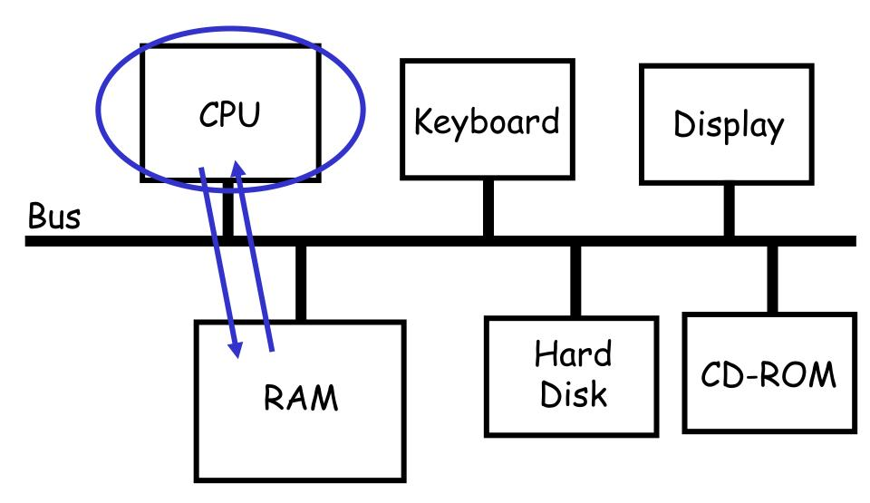
• This cycle is orchestrated by the Control Unit in the CPU.
