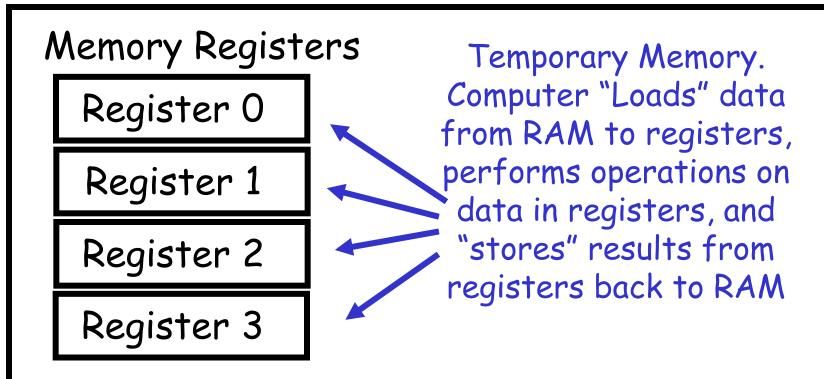
Remember our initial example: "read value of A from memory; read value of B from memory; add values of A and B; put result in memory in variable C." The reads are done to registers, the addition is done in registers, and the result is written to memory from a register.
